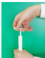
Handle to operate plug at end of sampler
