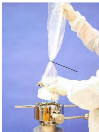
Attaching the two halves of the valve together
