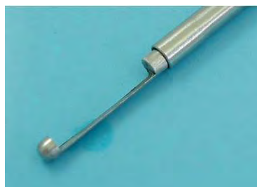
Sample tip can be easily adjusted to vary the volume of the sample taken
