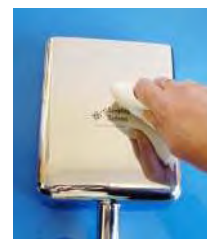
4. Clean etching area thoroughly using demineralised water
