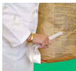
2. Insert the sampler through the side of the sack.
