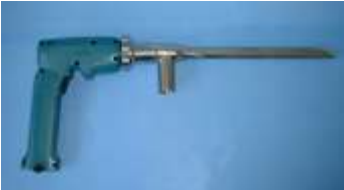
Horizontal Suitable for sampling horizontally. Particularly useful if sampling from sacks
