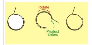
Rotate the inner core to open the sampler
